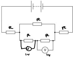
The reading on the voltmeter is 1.0 V.
